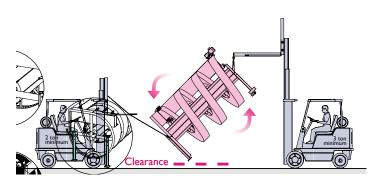
*Caution: ensure that all lifting equipment (slings, straps, eyes, etc.) are properly certified and secured before any lifting operation*
